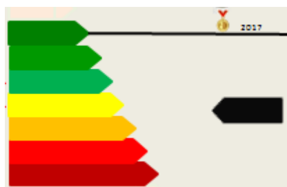
Figure 6 Illustrations of two ways of indicating where - in the ranking - the best available technology of a certain year is (line or green arrow plus symbol; the black arrow indicates the performance of the specific appliance as this is also indicated on the existing label)
